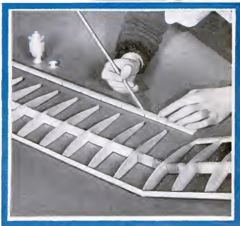
Constructing the wing. The slots cut in the trailing edge for the ribs are being coated with cement
